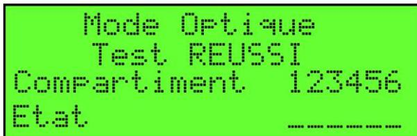
Optic pass when connected to an onboard monitor will show dashes for sensor status. Onboard monitors do not have a diagnostic connection to the rack monitor and do not pass the number of good sensors through the onboard monitor to the socket.
