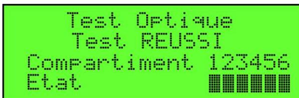
Optic pass when connected to sensors is shown above. A black square will light for each good sensor.
