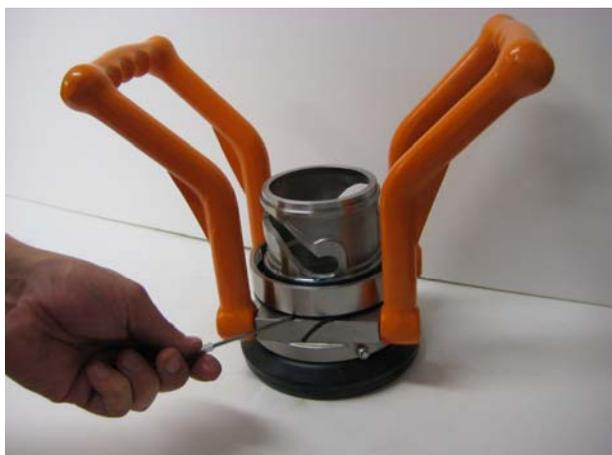
Change the O-ring (pos.24) from the groove in the coupling body. Use grease on the new part. Apply grease on the balls for best possible swivel rotation.
