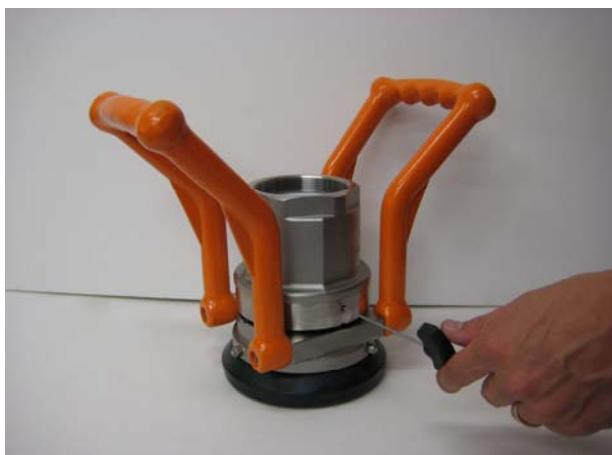
**Begin with unscrewing and remove the lock screw from the swivel ring.**
