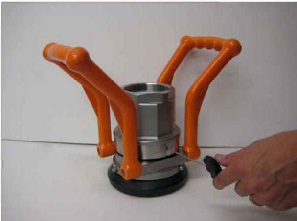
**Use Loctite® 243 and screw the lock screw into the swivel ring without any force! Risk to deform the ball bearing!**
