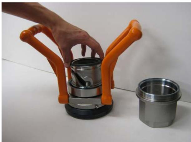
**Change the Teflon® ring (pos.25) on the top of the coupling body.**
