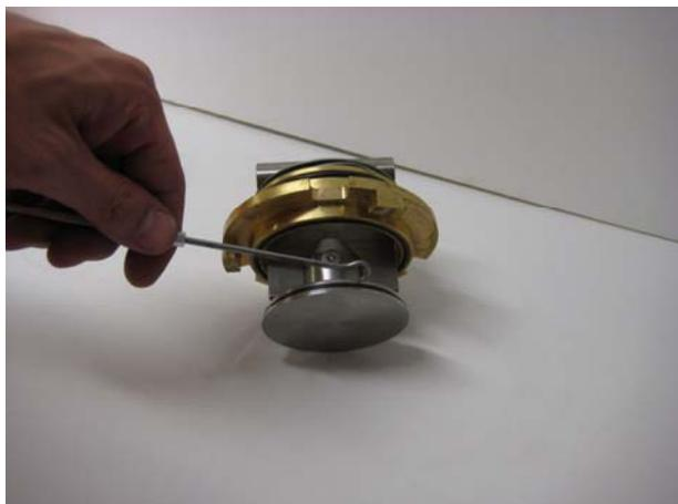
**Change the O-ring (pos.3) on the piston. Use grease on the new O-ring. Make sure that the O-ring doesn't get twisted when mounting.**
