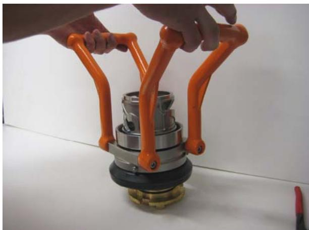
Turn back the unit and remove the driving plate packet from the coupling body.
