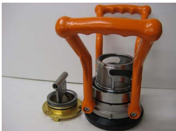
**Before the coupling body places on the driving plate packet, make sure that the part where the upper cam curve ends, shall be placed exactly over one roll, and the heel on the driving plate packet should be placed under the hole for the shaft.**
