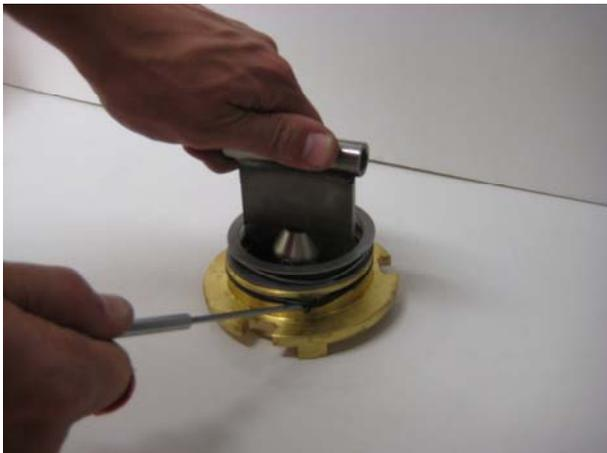
**Change the O-ring (pos.8) on the driving plate back side. Use grease on O-ring.**
