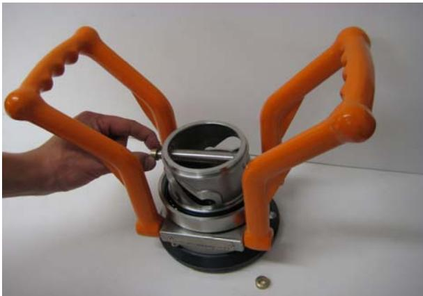
**Assemble the two shafts for piston guide.**
