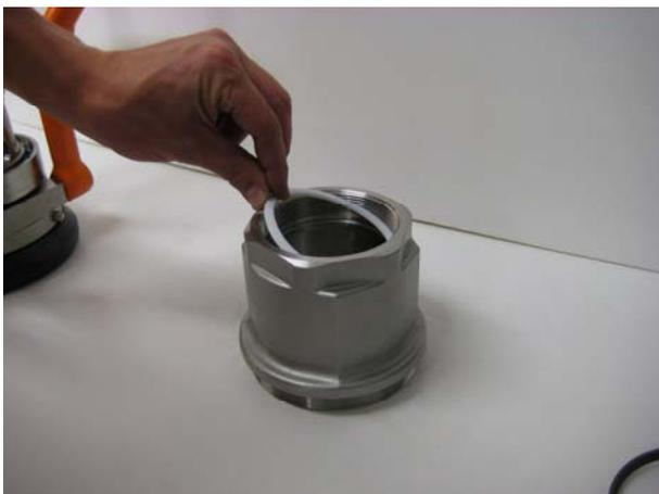
**Place a new flat seal (pos.29) on the swivel sleeve. (Not needed when NPT-thread)**
