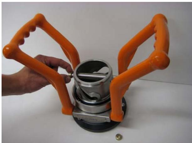
Remove the two rollers and the rolling shaft from the piston guide.
