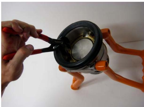
Turn the driving plate to the position where the recess ends up under the rollers under pressure to the driving plate packet.
