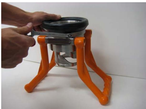
Change the three shafts (pos.18), locking nuts (pos.19) and rollers (pos.17) to new ones.
