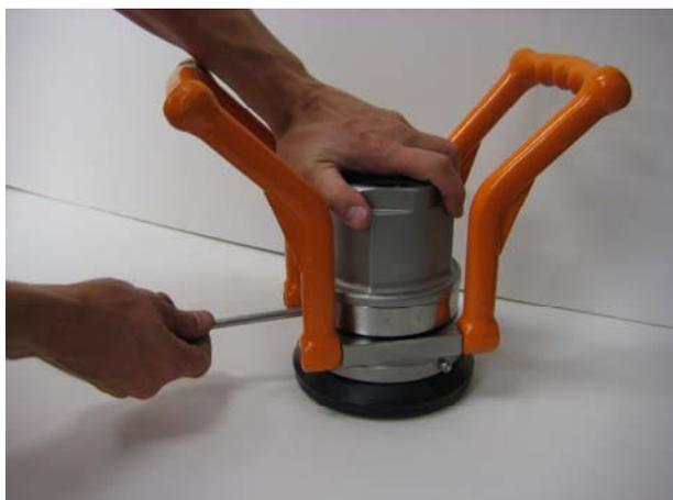
**Mark the position of swivel sleeve against swivel ring with an Ø8 mm pin.**
