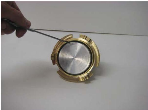
**Change the O-ring (pos.6) on the driving plate front side. Use grease on O-ring.**
