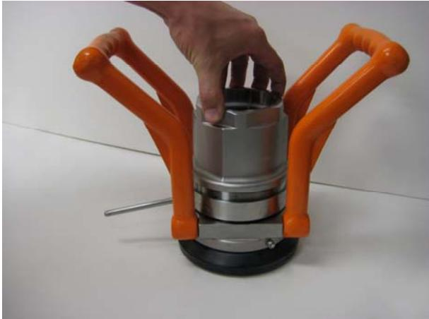
**Place the swivel sleeve over the coupling body and screw in the swivel sleeve.**
