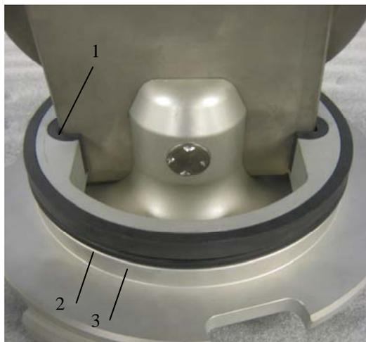
Change the O-ring (pos.8) and Teflon® ring (pos.9) on the driving plate back side. Use grease on O-ring.
