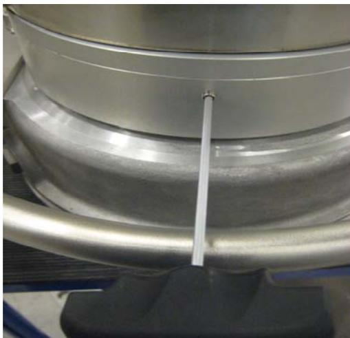
**Use Loctite® 243 and screw the lock screw into the swivel ring without any force! Risk to deform the ball bearing!**
