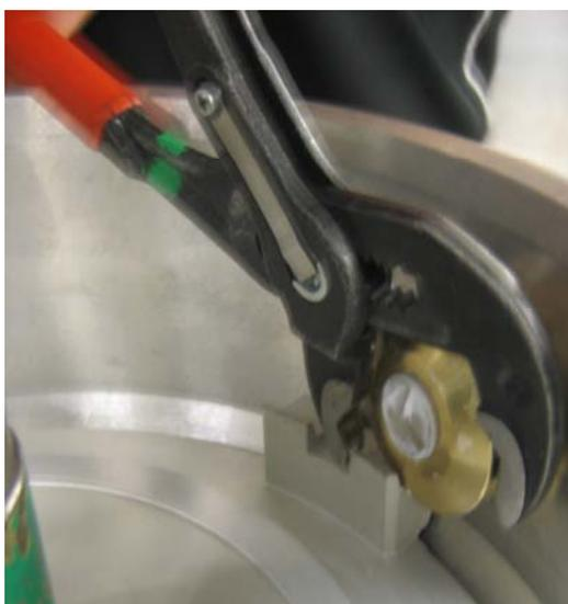
**Turn the driving plate to the position where the recess ends up under the rollers under pressure to the driving plate packet.**
