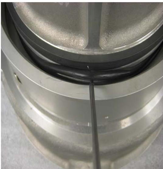
**Change the O-ring (pos.24) from the groove in the coupling body. Use grease on the new part. Apply grease on the balls for best possible swivel rotation.**
