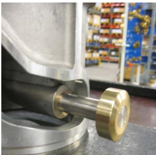
Assemble the two shafts for piston guide when applying pressure to the driving plate packet.
