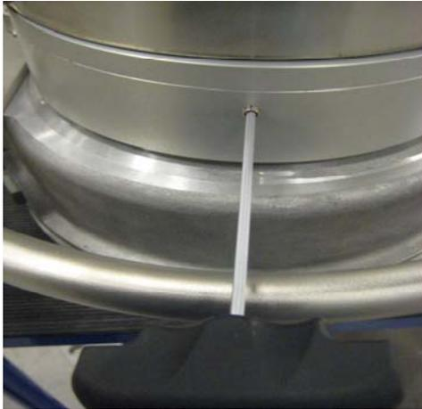
**Begin with unscrewing and remove the lock screw from the swivel ring.**
