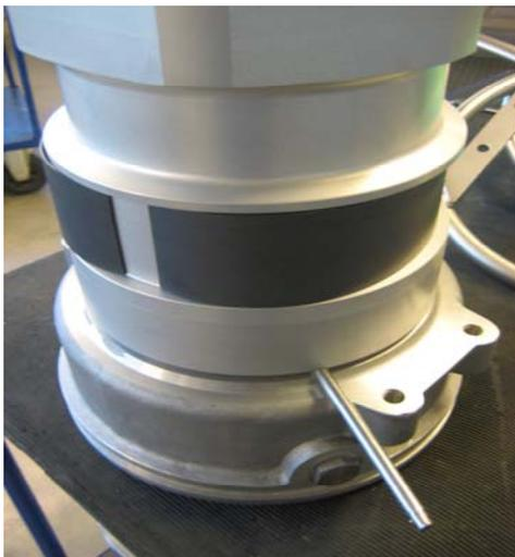
**Mark the position of swivel sleeve against swivel ring with an Ø8 mm pin.**
