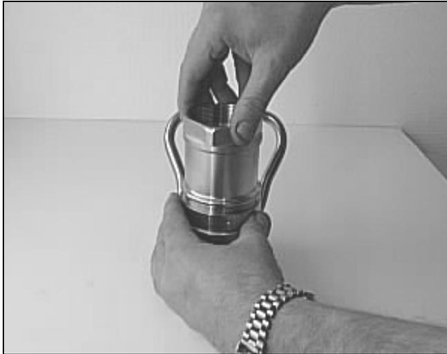
**Place the swivel sleeve over the coupling body and screw in the swivel sleeve.
