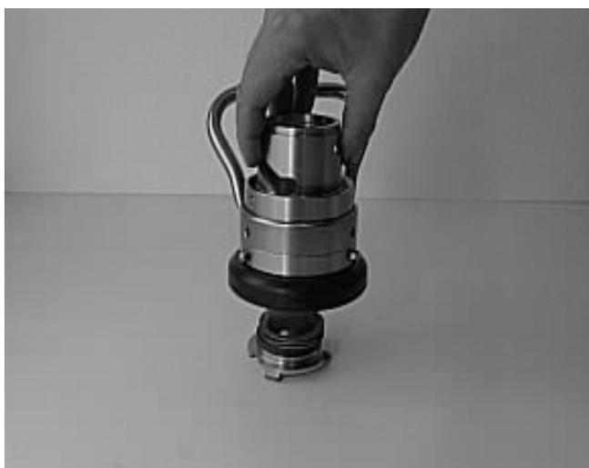
**Turn back the unit and remove the driving plate packet from the coupling body.**
