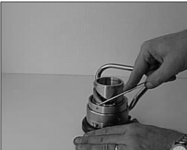
**Remove and change the O-ring (pos.24) from the groove in the coupling body.**
