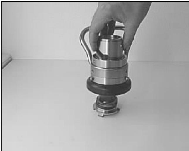
**Place the coupling body over the driving plate packet. Grab the piston guide and turn the unit upside down.**
