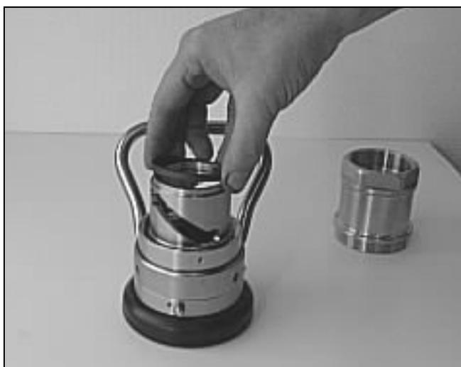
**Remove the Teflon® bushing on the top of the coupling body.**
