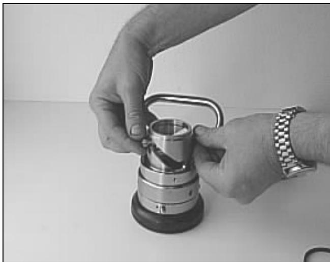
**Assemble the two shafts for piston guide.**
