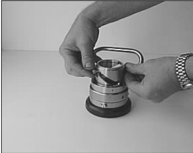
**Remove the two shafts for piston guide and the two cylinder Teflon® bushing**
