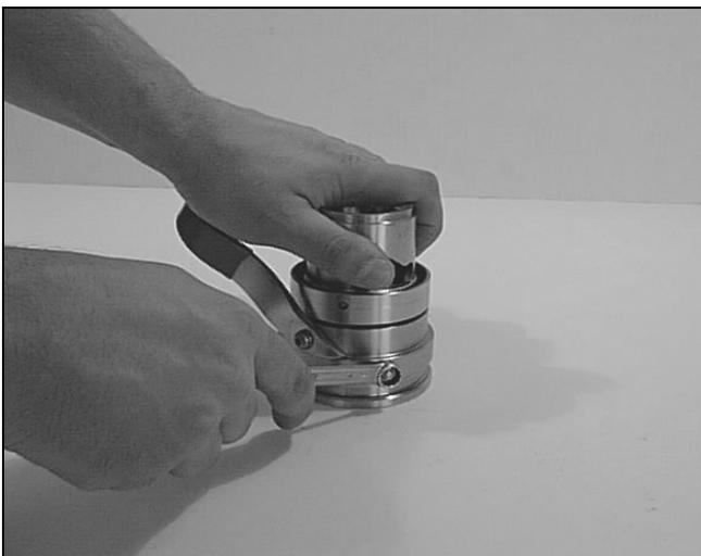
**Change the three shafts (pos.18), locking nuts (pos.19) and rollers (pos.17) to new ones.**
