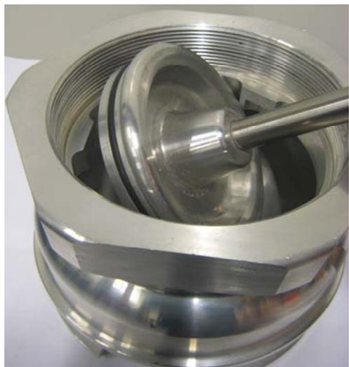
**To take out the piston put into a relaxing position in the valve seat.**
