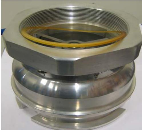
**Remove the flat sealing.**
