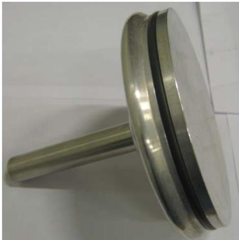
**Replace the O-ring (pos.3) on the piston with a new greased O-ring.**
