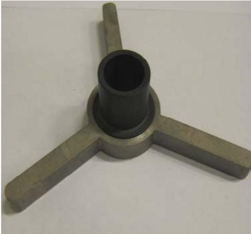
**Replace the Teflon® bushing (pos.5) in the spindle steering with a new one.**
