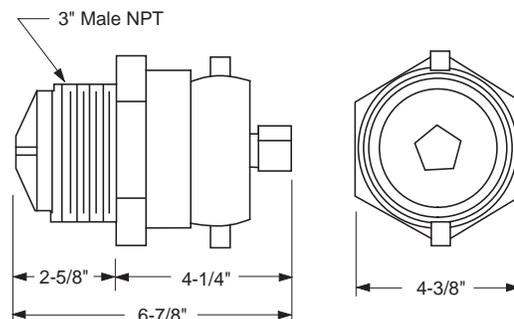
NOTE: Under no circumstances should a check snoot be installed directly into a pipe, as this may prevent the snoot from opening. Install directly into the appropriate standpipe body only.
