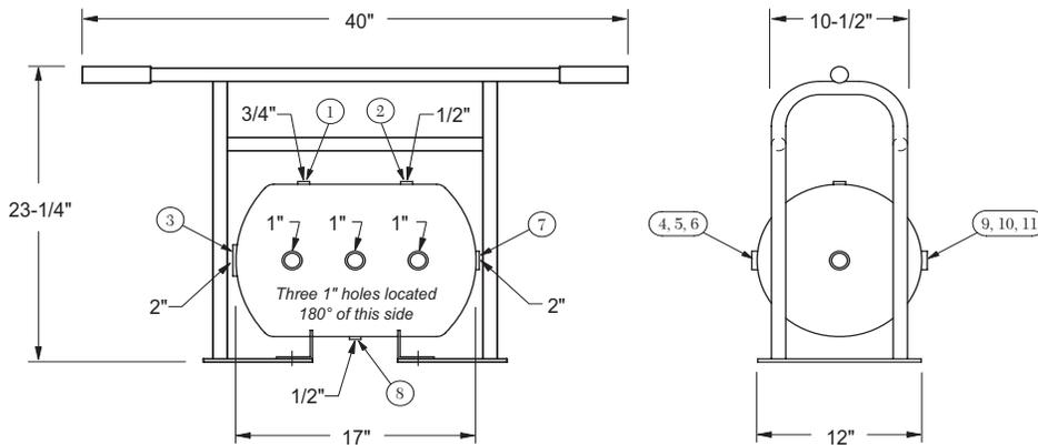
Dixon® 1217AR-4AK air receiver manifold assembly with Air King® outlet ports includes the following components:
