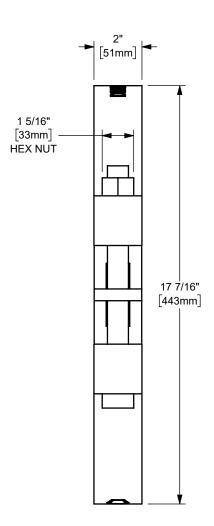
HOSE OD RANGE: 15 4/64" [382.6mm] - 17 32/64" [444.5mm] TORQUE: 200 ft. lbs. [271Nm]
