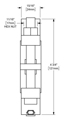
HOSE OD RANGE: 3 32/64" [88.9mm] - 3 52/64" [96.8mm] TORQUE: 40 ft. lbs. [54Nm]
