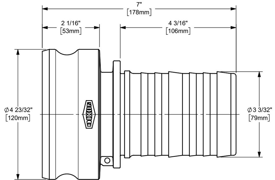
MAX PSI WHEN HOSE IS ATTACHED WITH A KING CRIMP FERRULE OR SLEEVE: 150 PSI
