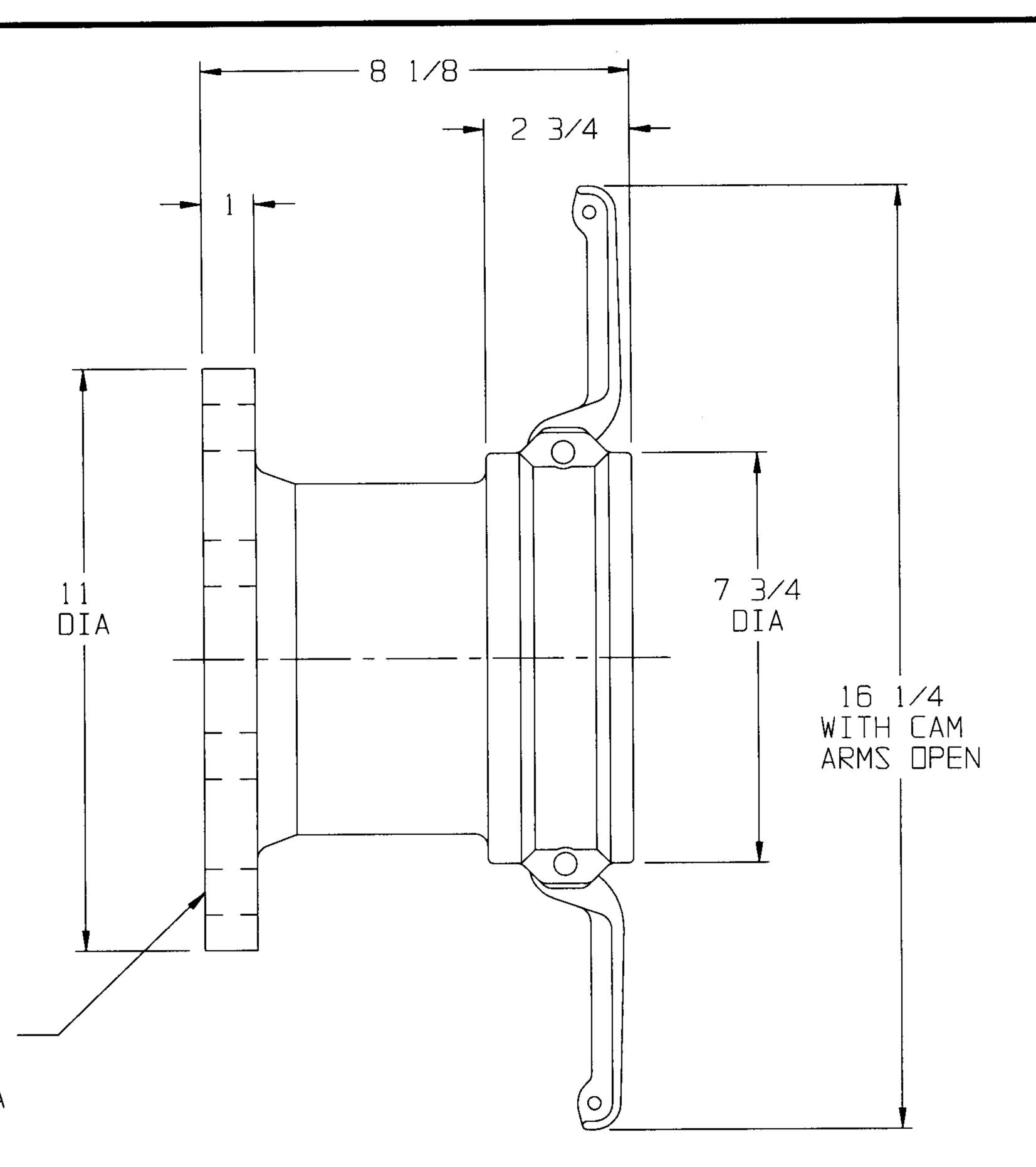
7/8 DIA TYP 8 HOLES EQUALLY SPACED ON A 9 1/2 BOLT CIRCLE DIA
