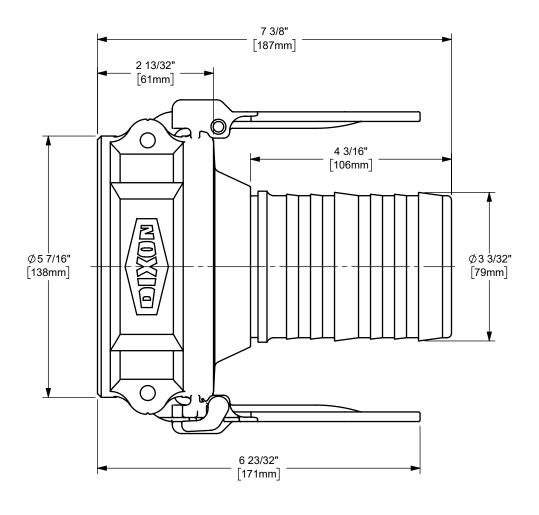
DISTANCE ACROSS OPEN CAM ARMS: 16 5/8" MAX PSI WHEN HOSE IS ATTACHED WITH A KING CRIMP FERRULE OR SLEEVE: 150 PSI MAX PSI WHEN HOSE IS ATTACHED WITH BAND CLAMPS: 100 PSI
