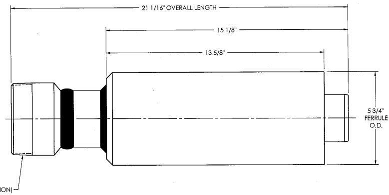
4" ÁPI LINE PIPE THREAD SPEC 5B (MOST CURRENT EDITION) —
