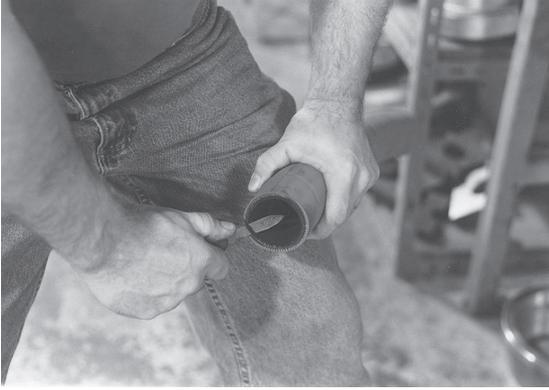
Assuring that the hose end is cut square, chamfer the I.D. of the hose  $\frac{1}{8}$ " at a 45° angle. This will aid in stem insertion. If the hose is to be static grounded, follow hose manufacturers procedure for proper static grounding.
