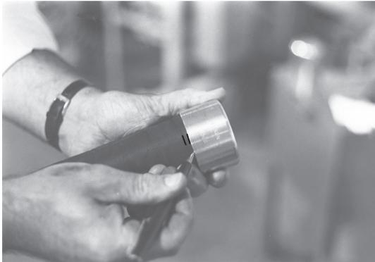
Make sure the hose end is cut square. Slide the ferrule over the hose until the turned over end of the ferrule contacts the end of the hose. Place a mark on the hose at the junction of the ferrule and hose. Move the ferrule away from the hose end  $\frac{1}{8}$ " and place another mark at the junction of the hose and ferrule. This will insure that the proper rubber displacement or pocket is maintained during the expansion process.
