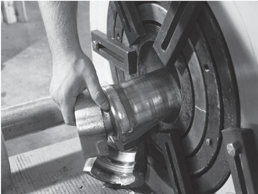
Reposition the tie down bars on the die face so that the wing nut (or spacer) will clear.
