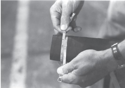
Accurately measure the hose O.D. with a diameter tape. Select the correct Holedall™ Petroleum Ferrule from the DPL based upon the Hose O.D. just measured.
