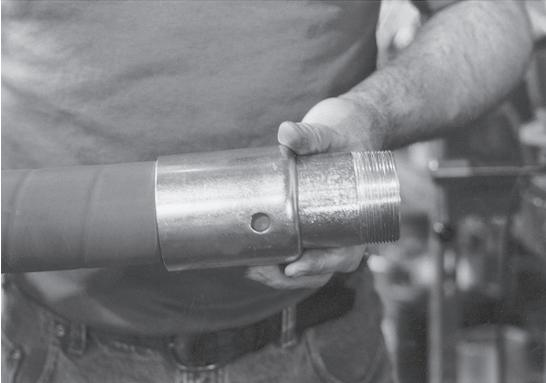
Slide the ferrule over the stem and over the O.D. of the hose until the turned over portion of the ferrule rests on the ring of the stem.
