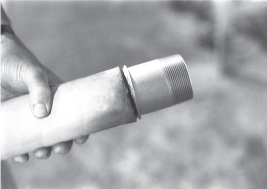
Lubricate the I.D. of the hose and the O.D. of the stem with Dixon Coupling Lubricant or equivalent. Insert the stem into the hose until the hose end contacts the stem collar. Position the sight hole on the ferrule so that this can be observed. After stem insertion, slide the ferrule down until the turned-over part of the ferrule contacts the stem collar.
