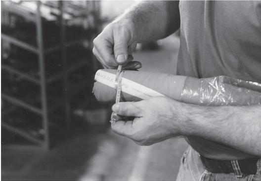
Accurately measure the hose O.D. with a diameter tape. Select the correct IX ferrule from the current Dixon Price List based upon the hose O.D. just measured.
