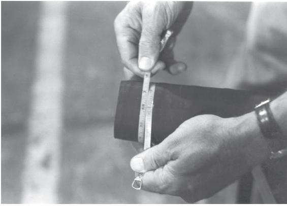
Accurately measure the hose O.D. with a diameter tape. Each end of the hose should be measured to guarantee the correct ferrule and die selection. Select the correct ferrule and die based upon the hose free O.D. just measured from the die chart. Make sure that the hose end is cut square. If the hose is to be static grounded, follow hose manufacturers procedure for proper static grounding.
