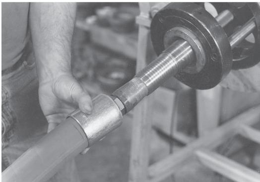
Slide the hose with the ferrule on over the IX plug and shank until the ferrule contacts the shoulder of the stem. Make sure you align the ferrule with the second mark from Step 8. Make sure the pocket has been maintained.
