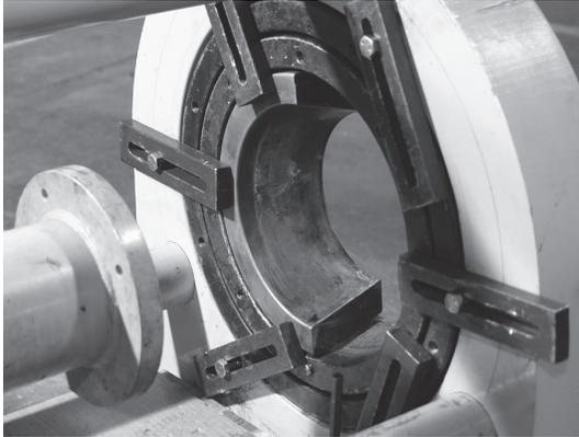
Position a rubber sheet or pad under the die bed. While holding the die in place with one hand, loosen the bolt on the tie down bar and move the tie down bar so that it clears the die. Slowly slide the hose towards the pusher. When the die clears the die holder, one or both halves may fall to the floor. If one half remains on the ferrule, tap it with a mallet until it releases. If both halves remain on the ferrule, it may require the halves be pried apart at the seam.
