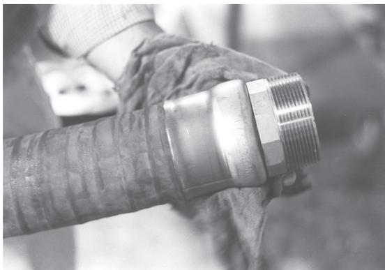
Lubricate the O.D. of the stem and the I.D. of the hose with Dixon lubricant or equivalent. Insert the end of the fitting into the hose. Assemble the ferrule onto stem by sliding turned over portion of ferrule past notched section of stem collar. Rotate ferrule 90° ( $\frac{1}{4}$  turn). With ferrule and stem engaged, continue installing stem until ferrule reaches the second mark on the hose.
