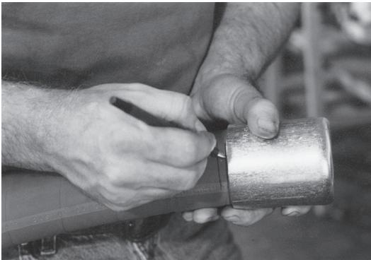
Make sure the hose end is cut square. Slide the ferrule over the hose until the turned over end of the ferrule contacts the end of the hose. Place a mark on the hose at the junction of the ferrule and hose. Move the ferrule away from the hose end  $\frac{1}{4}$ " and place another mark at the junction of the hose and ferrule. This will ensure that the proper rubber displacement or pocked is maintained during the expansion process.
