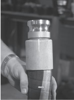
Check the ferrule for proper alignment. Ensure that the mark on the ferrule (from Step 6b) is in the center of the stem collar.
