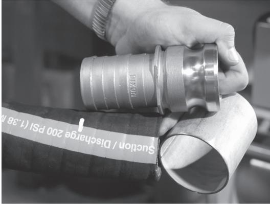
Align the end of the hose with the stem shoulder and mark the hose at the end of the stem
