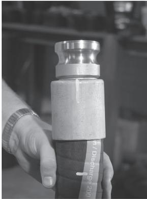
Place a mark on the outside of the ferrule that corresponds with the center of one of the turned over sections of the ferrule. This mark will act a guide for correct engagement with the stem collar.
