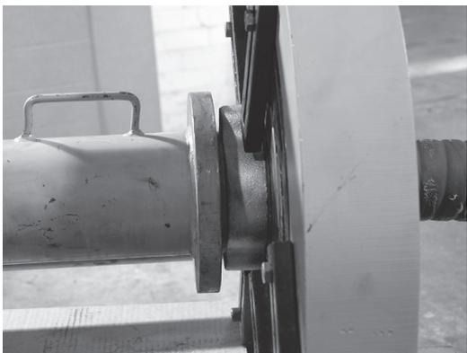
Depress and hold the button on the remote until the wing nut (or spacer) contacts the die face. Release the button. Return the directional control lever to the "NEUTRAL" position.
