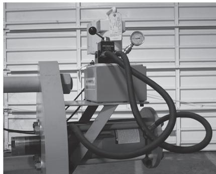
Caution! Never dead-end the cylinder (fully extended or fully retracted) and leave it with pressure showing on the gage. If the cylinder is dead-ended, always move the lever to the neutral position after stopping the pump. Failure to do so can shorten the life of the cylinder seals.
