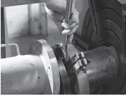
Extend all of the jackscrews so that they are contacting the flange. With a wrench, tighten one jackscrew one half turn. Moving to the jackscrew opposite of the one just tightened, tighten it one half turn. Moving to the jackscrew immediately to the right of the first one tightened, tighten it one half turn. Moving to the jackscrew opposite of the one just tightened, tighten it one half turn. Keep repeating this process until all jackscrews are evenly tensioned.
