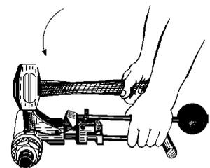
*Instructions for using adapter to apply 3/8" width clamps*
