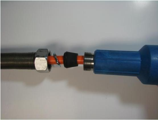
Per the picture above, slide the new rack cord through the strain relief spring and nut, then through the metal backup ring and rubber grommet and through the rack plug body.
