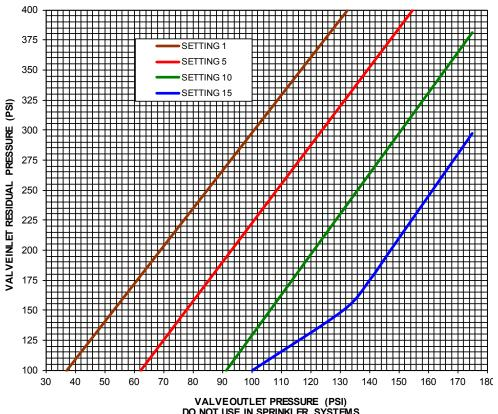
VALVEOUTLET PRESSURE (PSI) DO NOT USE IN SPRINKLER SYSTEMS WITH OUTLET PRESSURE BELOW 50 PSI
