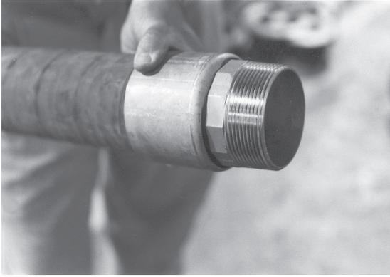
Lubricate the O.D. of the stem and the I.D. of the hose with Dixon lubricant or equivalent. Insert the end of the fitting into the hose. Assemble the ferrule onto stem by sliding turned over portion of ferrule past notched section of stem collar. Rotate ferrule 90° (¼ turn). With ferrule and stem engaged, continue installing stem until ferrule reaches the second mark on the hose.
