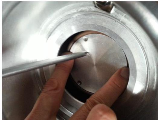
12. Install the cage (2) to the poppet (3) using the machine screws (6) and washers (20).
