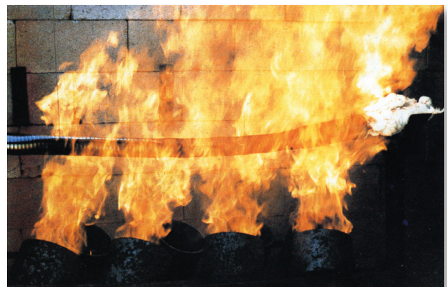
GSM BOP hose tested at 2,000°F (1093°C) (2,000,000 BTU's) at 5,000 PSIWP.
