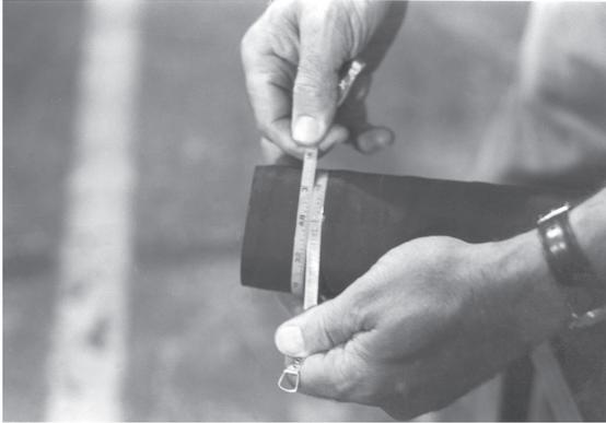
Accurately measure the hose O.D. with a diameter tape. Each end of the hose should be measured to guarantee the correct ferrule and die selection. Select the correct ferrule and die based upon the hose free O.D. just measured from the chart.
