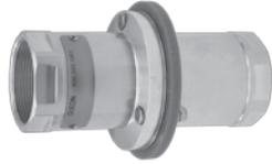
The typical applications for these couplings are ship-to-offshore platform and ship-to-ship product transfer operations. These couplings are made from 316T1 stainless steel and have Viton® O-rings. The industrial and marine couplings are available in Female NPT, Male NPT, and Flange connections.
