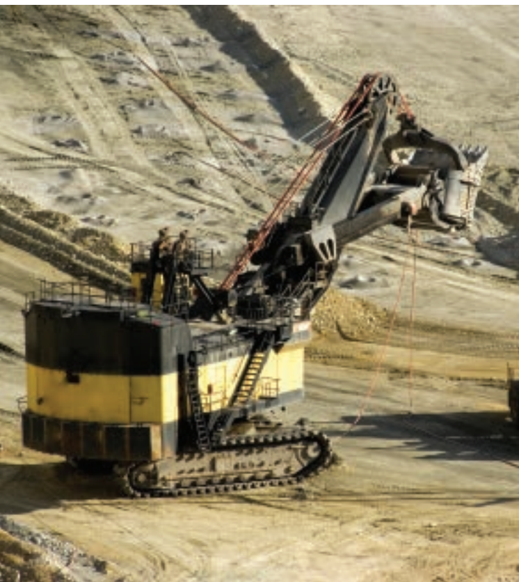
Left to right: A mine with a hand-dirt machine; a giant electric shovel that can scoop 98 tons of ore per shovelful; copper sulphide slurry pours from a machine in a processing facility at Katanga Mining Ltd.'s copper and cobalt mine in Kolwezi.
