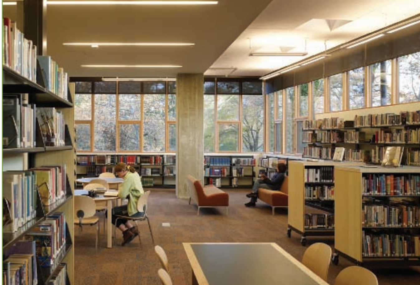
Sidwell Friends Middle School's library allows sunlight to permeate the room. Virtually all interior spaces receive some daylight. Elsewhere in the school, thermal comfort is enhanced and energy use is reduced through the use of ceiling fans, which allow air-conditioning temperatures to be comfortably set 5 degrees warmer than usual.
