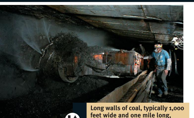
Left: A continuous miner cutting coal Above: A long-wall miner shearing coal
