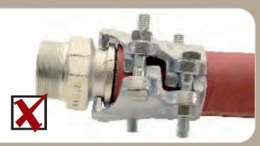
arms from opening while loading. New employees were instructed, in addition to use of proper safety gear, to attach the coupler to the adapter on the tank car, then insert a wire through the rings on the cam arms. twist the wire until the cam arms were secured in the closed position, and then start the pump.
